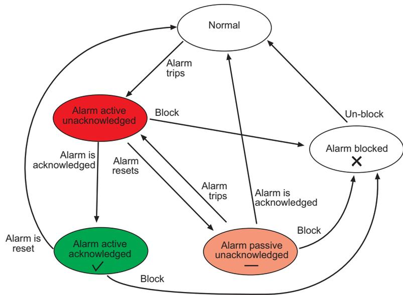
Fig. 4.8: Alarm state transitions.
